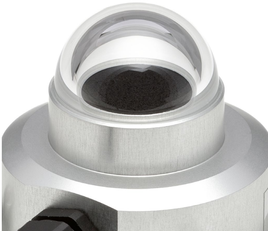
Figure 0.2 SR03 fast response second class solar radiation sensor
