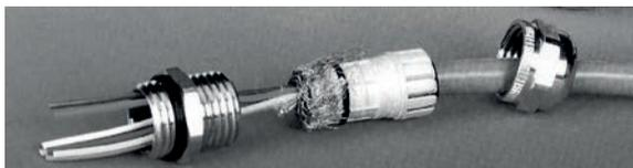
The braided screen should be turned back via the plastic insert on the cable connection. The introduction of the plastic insert presses the braided screen onto the interior wall of the metallic part.
