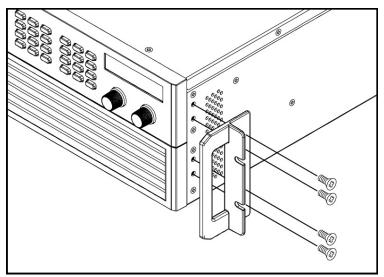
Figure 2-9 Installing the Handle
