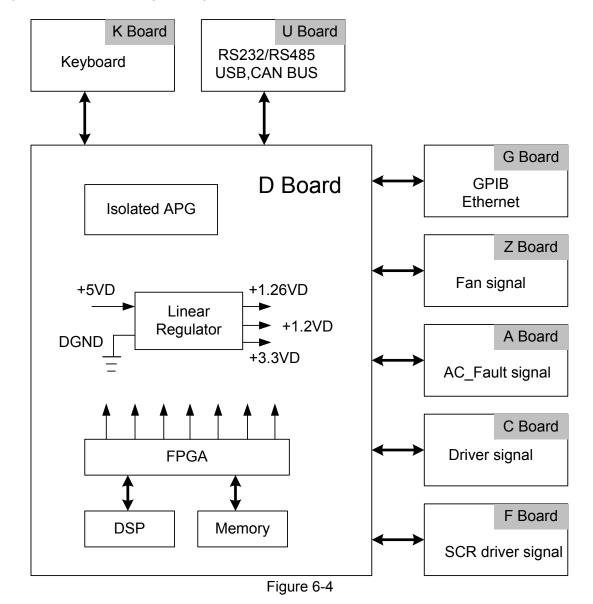
Figure 6-4 shows the digital stage structure.
