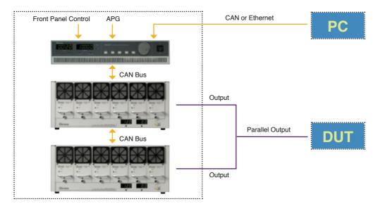
Type B - Control without CSU: User can only control via CAN Bus for paralleled operation.
