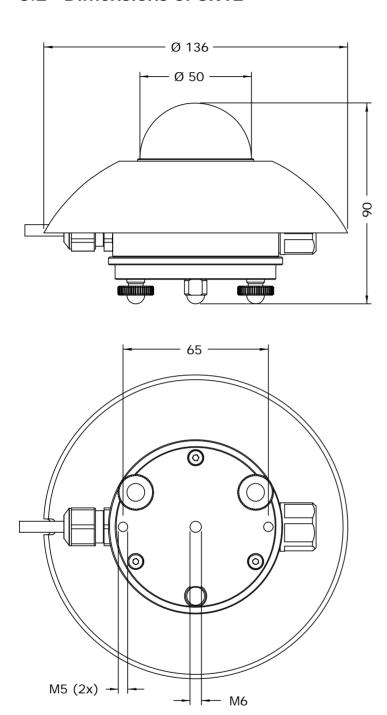
**Figure 3.2.1** Dimensions of SR12 in 10<sup>-3</sup> m.
