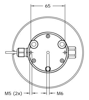
Figure 8.2.2 Dimensions of SR12-TR in 10<sup>-3</sup> m
